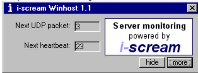
Clicking on "Hide" causes the dialogue to disappear. Clicking on "More" expands the window to provide you with information about the data being sent to the filter or filter manager and gives you the option to force the WinHost to reconfigure with the filter manager.
