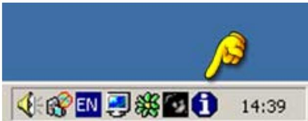
Double-clicking on this icon brings up the WinHost interactive dialogue. This shows the number of seconds left until a *UDP* packet is sent to the filter machine and the number of seconds until a *heartbeat* occurs with the filter machine.
