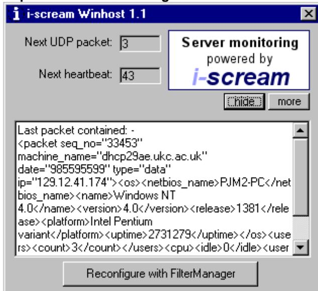
When the WinHost is started, it attempts to obtain its configuration from the filter manager. Progress through this stage is displayed in the large text area if the WinHost is running in Expanded mode. It will display the information received from the filter manager as it receives it. This output includes details such as the address of the filter machine that the WinHost will use.
